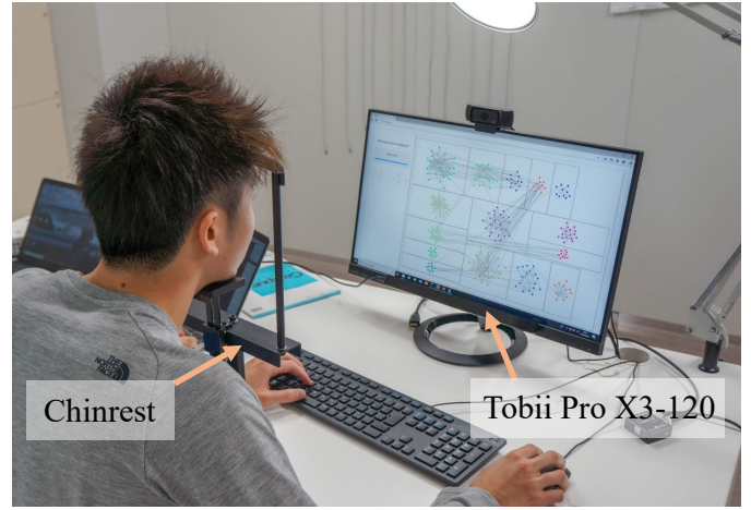
Fig. 5. Experimental environment. The eye movement was recorded using an eye tracker attached to the bottom of the monitor.
